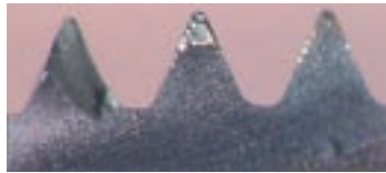
従来品 10穴加工後 Conventional after threading 10 holes.
