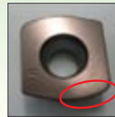
20分切削後の刃先摩耗写真 Photograph of flute wear after 20 minutes of cutting
