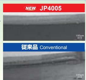
20分切削後の刃先摩耗写真 Photograph of flute wear after 20 minutes of cutting
